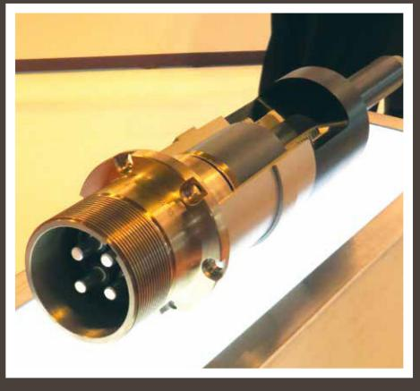
To eradicate the potential failure point at the cable and connector interface, specialist injection moulding processes are used to achieve chemical bonding to gland stems, connector shells, etc, whilst amalgamation of the jacket to the injected material retains all the strength and viscous elasticity without an adhesively based leak path.
